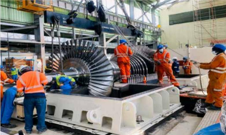
83.3 MW Olkaria Unit 6 turbine rotor assembly
